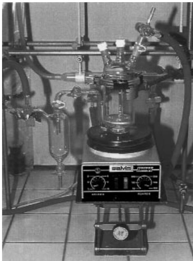
**Figure 1.** Photograph of apparatus setup as it is used (cooling bath removed to show more detail). The reaction mixtures are drawn off into the collecting funnel (left) and drained into a conical flask below.
